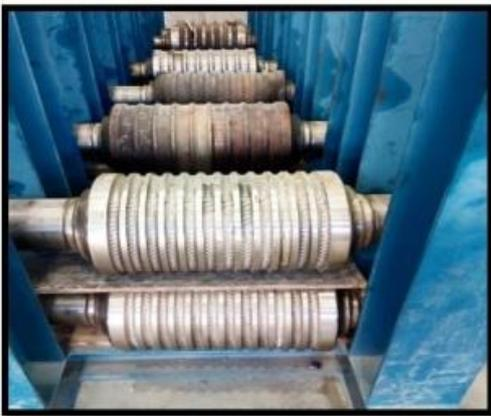
Figure I-16: Cylindres de laminage [29].
