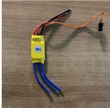
Figure III. 8 Electronic Speed Controllers (ESC 30A)
