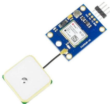
Figure III. 6 NEO-6M (GPS Module)
