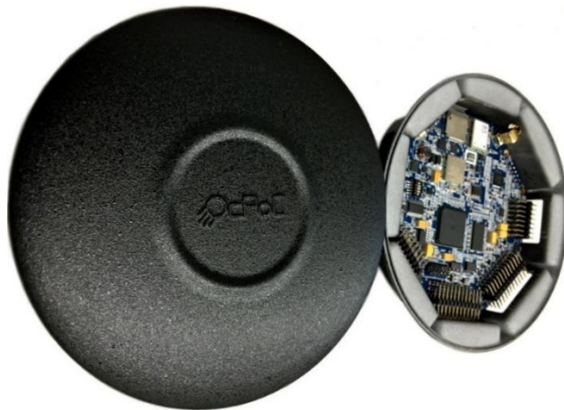
Figure II. 7 OCPOC (Octagonal Pilot on Chip) Flight Controller[14]
