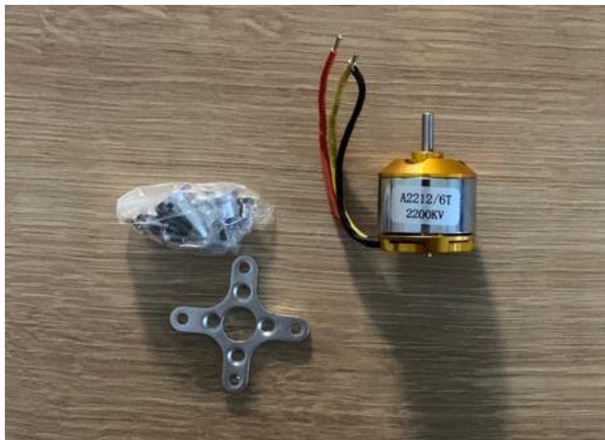
Figure III. 7 Brushless DC Motors (A2212/6 - 2200Kv)
