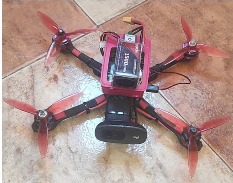
Figure 4.16. System's deployment on the drone
