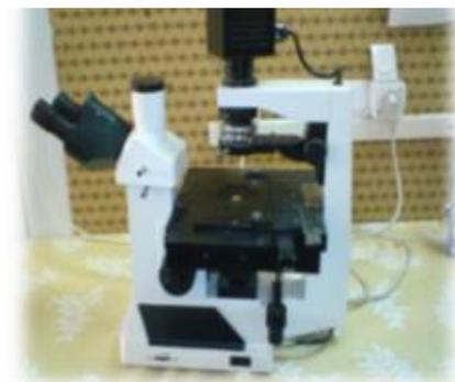
Fig.6: Microscope inversé
