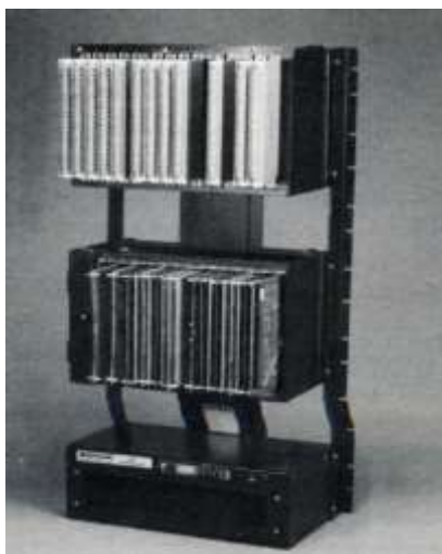
Figure 2.1 Automate programmable industriel (MODICON 084).
