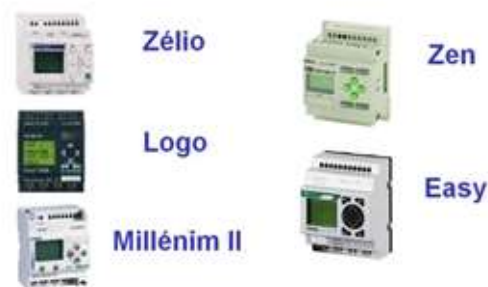
Figure 2.3 Les Modules compacts.[2]
