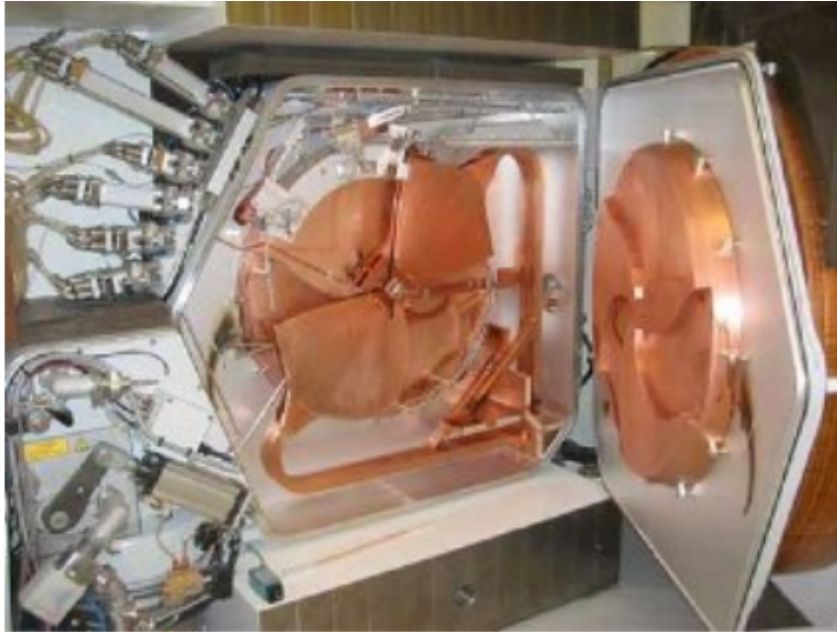
Figure 1.6: PETtrace cyclotron with internal ion source
