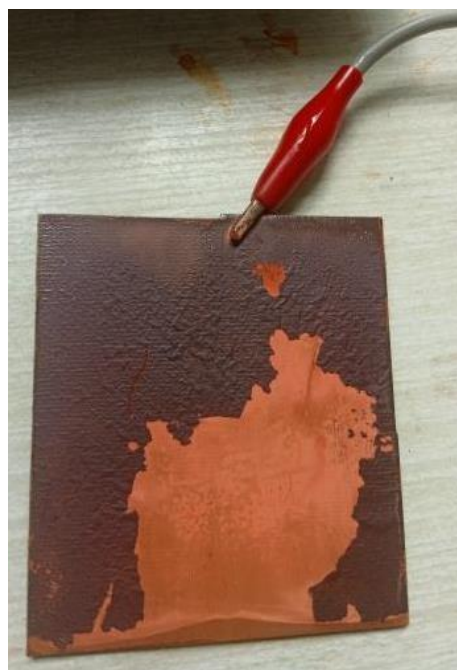
Figure II.16 Corrosion of copper piece
