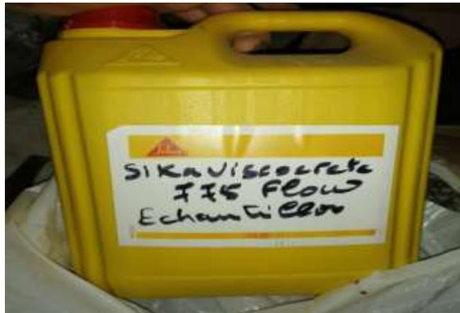
Figure IV.3. Adjuvant "Super-plastifiant Sika Visco-crete. [32]
