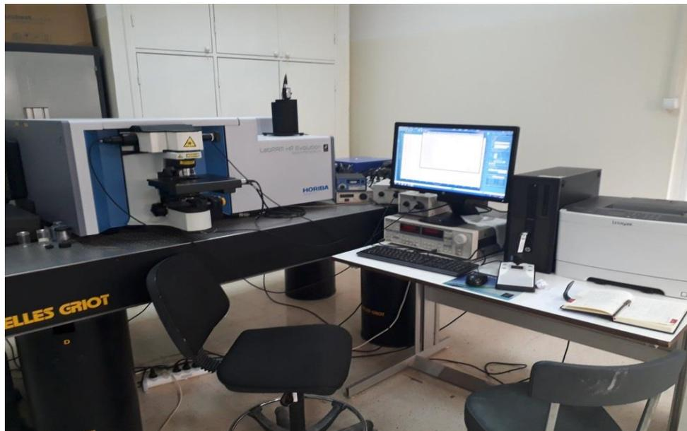
**Figure III-6:** Raman spectroscopy (CDTA).
