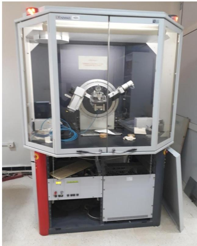
**Figure III-2:** Diffractometer D8 Advance Brucker (CDTA).
