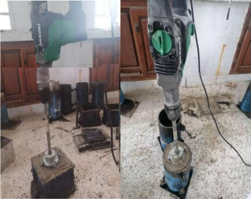
Figure.21: compactage de béton BCR
