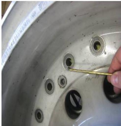
Figure II-II.5 Area of the bolt washers (scan circularly and radially to cover all possible cracks directions)
