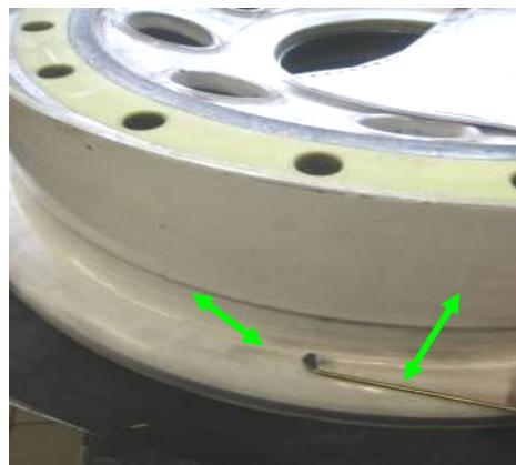
Figure II-II.2: **BEAD SEAT AREA** with scanning direction (twice at 90°) to cover the whole possible cracks directions
