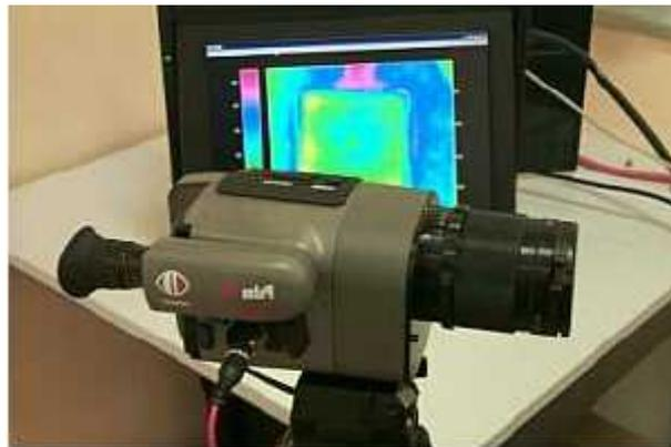
Figure 1-10 Camera infrarouge
