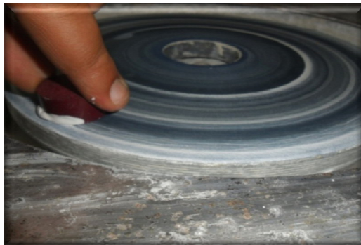
Figure III.16: 2 ème Etape de Polissage (Finition).
