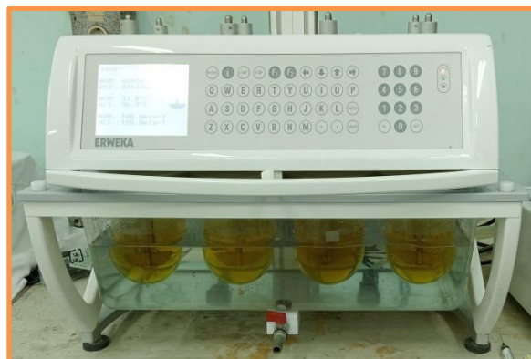
Figure III. 8: Le dissolutest (Photo originale)
