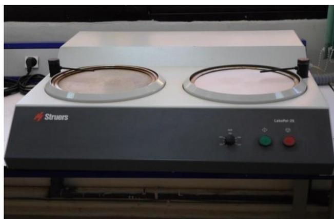
**Figure III.6:** Polisseuse Struers.
