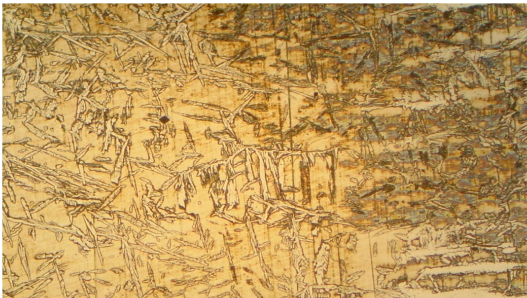
Figure III.10: Microstructure la ZL de acier (2205) GX200
