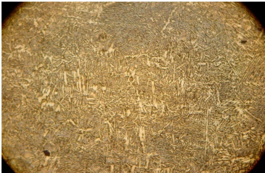
Figure III.8: Microstructure la ZF de acier (2205) GX200
