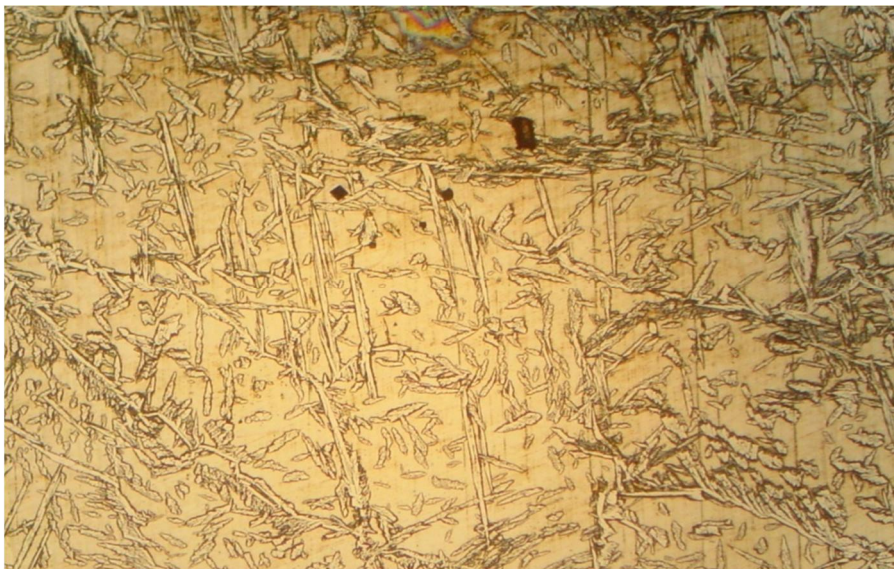
Figure III.6: Microstructure la ZAT de acier (2205).GX200
