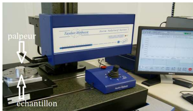
Figure III.6: Profilomètre de type Taylor Hobson Talysurf 120.
