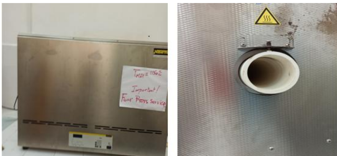
Figure III.6 Four tubulaire de frittage
