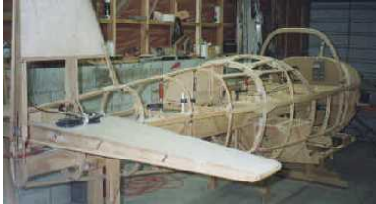
Figure ( II-5) La structure semi- monocoque
