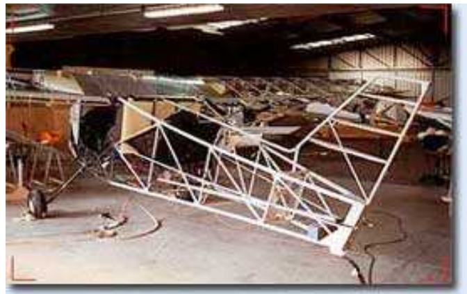
Figure ( II-4) La structure treillis
