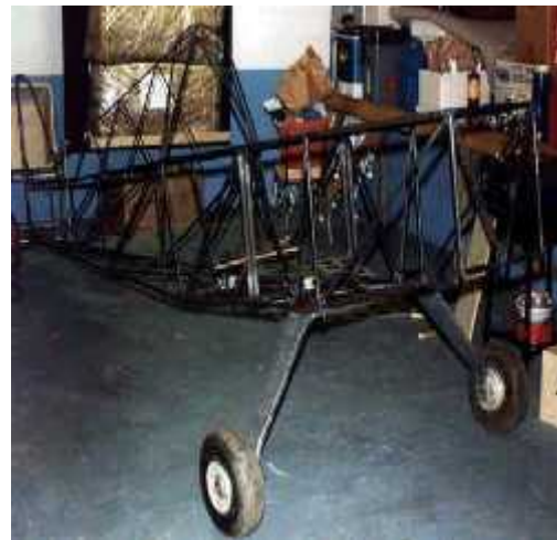
Figure (I-13.b) Structure métallique
