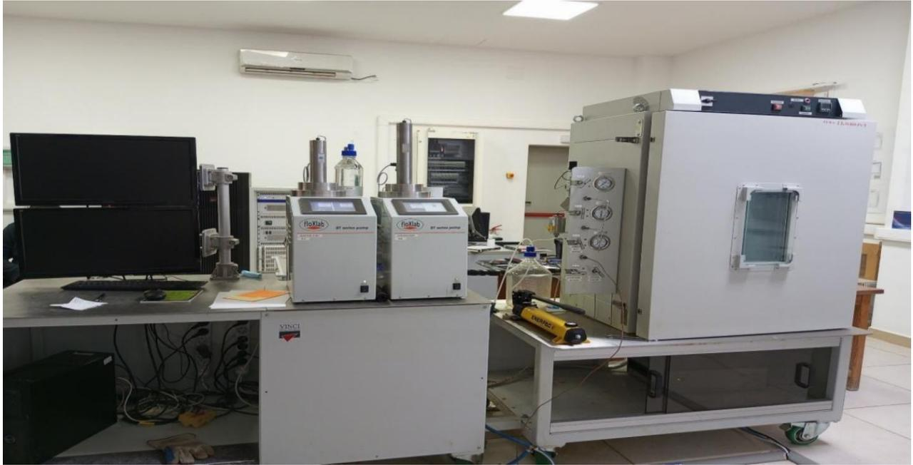
**Figure 3.3.** Core Flooding System CFS 350.
