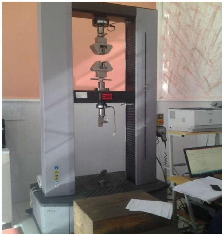
Figure III-3: Machine de traction (MTS) :
