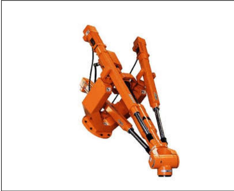
*Figure I-3: Robot parallèle*
