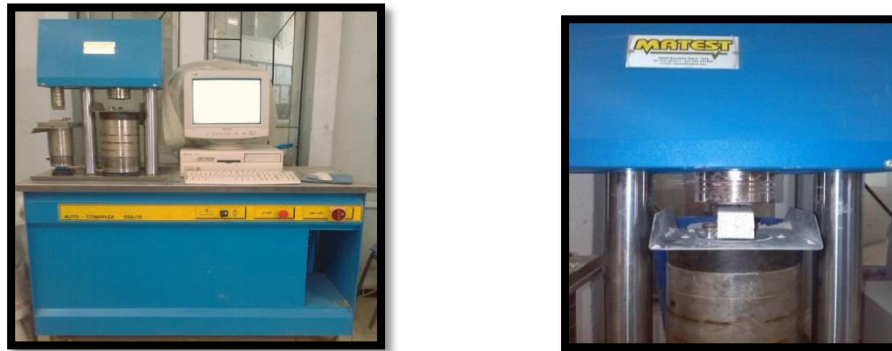
Figure II.11. La machine de compression.
