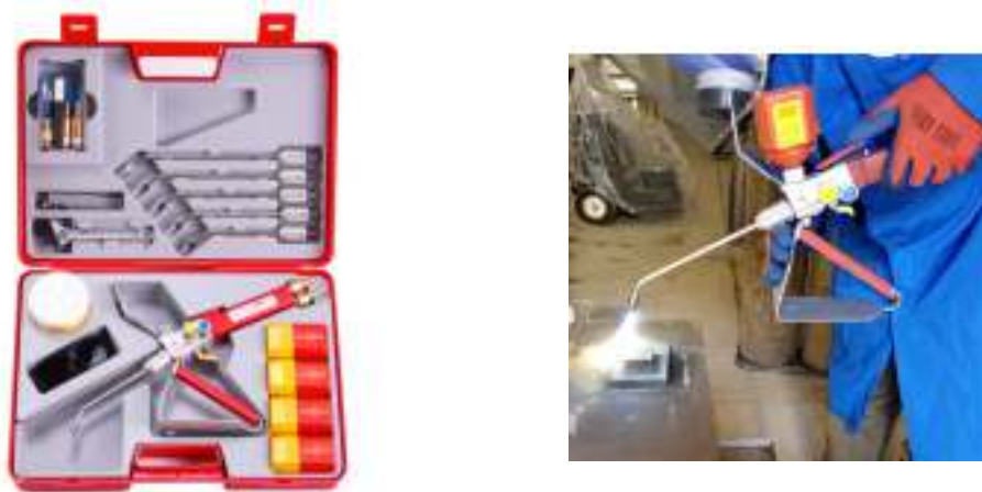
Figure 23 : Pistolet a flamme-poudre " kit Eutalloy "
