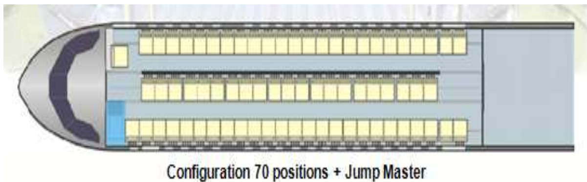
(fig I.4). Cabine passagers (transport passagers)
