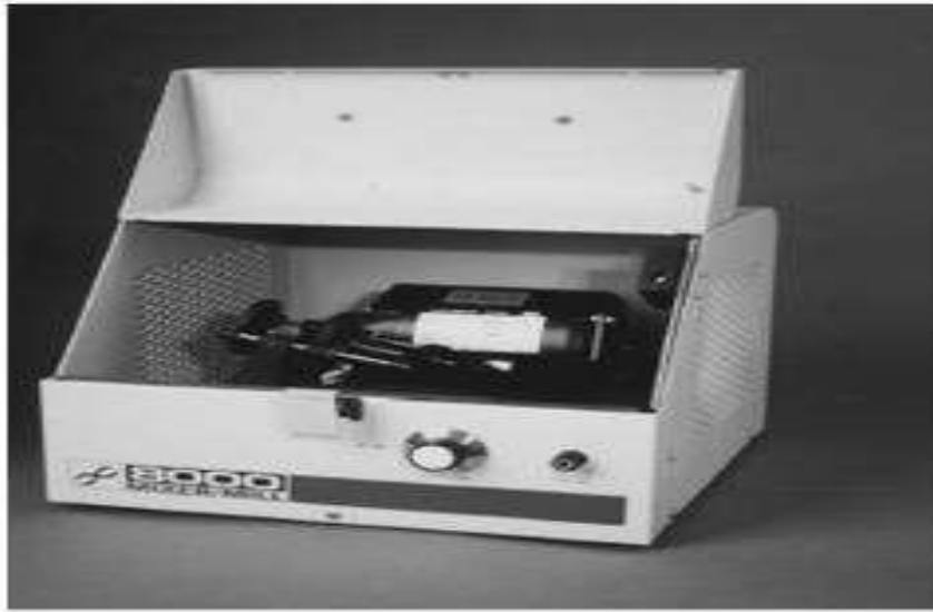
Figure 1. 9: broyeur vibratoire type SPEX 8000.
