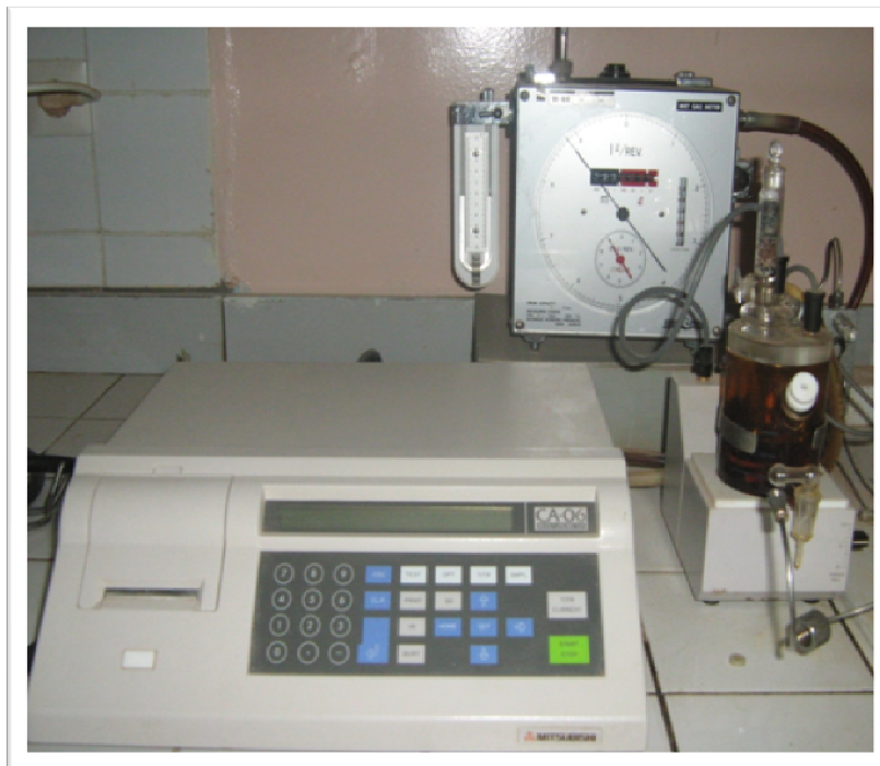
Figure III.2: Appareille de Karl Fischer
