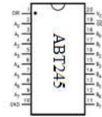
Fig.III.14 Brochage du composant 74HC 245.
