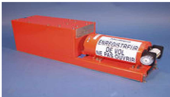
Figure (I.1): Le FDR "Flight Data Recorder"
