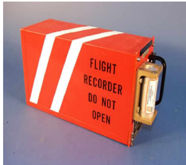
Figure (I.2) : Le CVR "Cockpit Voice Recorder"
