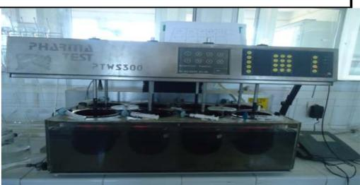
A photograph of a Pharma Test PTWS 300 Dissolution Tester. The instrument is black and has a control panel with a digital display and buttons.                        |
