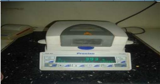
A photograph of a Precisa IR Desiccator. The instrument is white and has a digital display and buttons on the front.                                                 |
