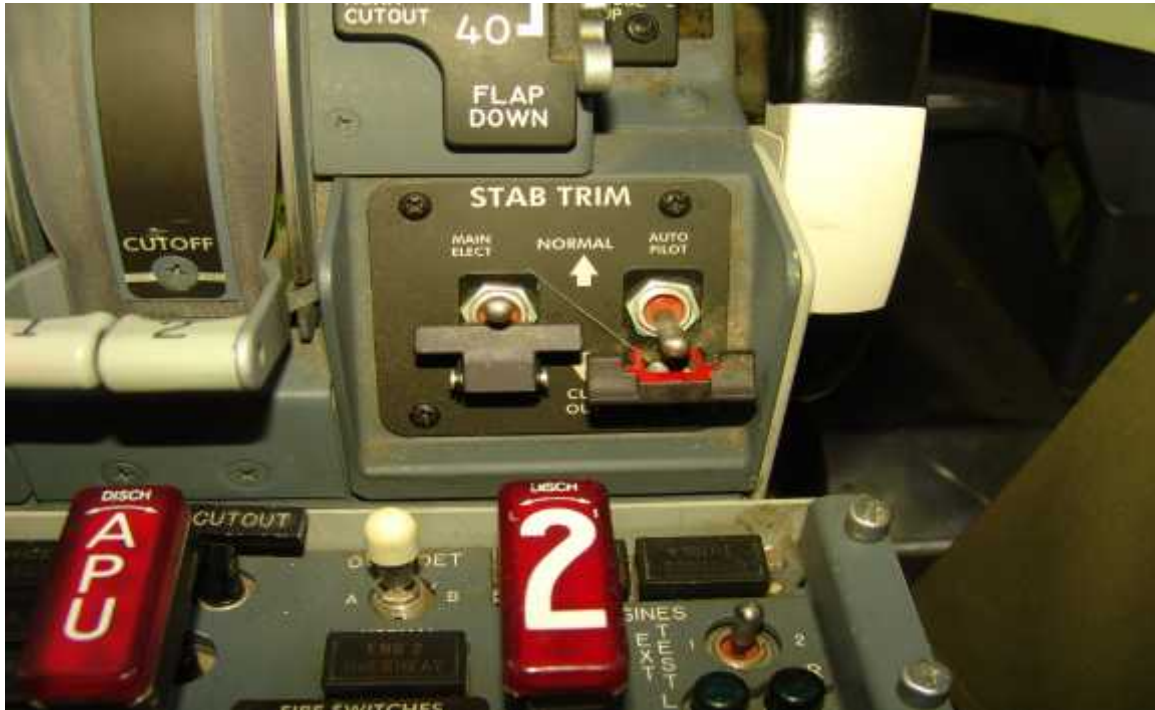
Figure (VI-3) : le stab trim cutout switch
