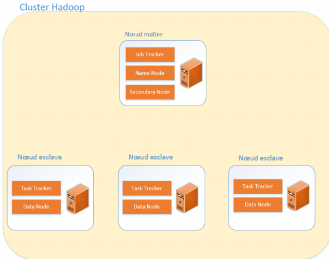
Figure I.8 : Architecture d'un cluster Hadoop[11]
