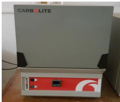
Figure. II-6. Four a moufle de type CARBOLITE
