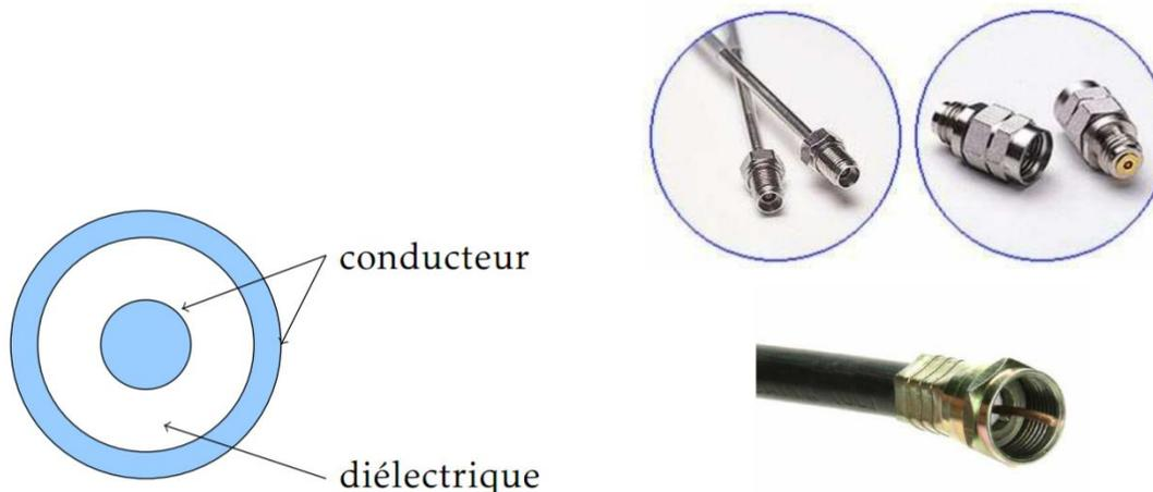
Figure 4.7 : Câble coaxial
