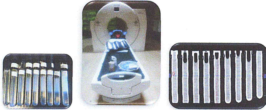
Figure III.4. Gel vials imaging with CT (Siemens®) scanner
