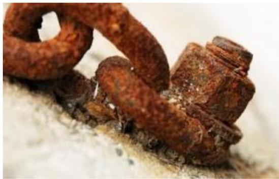
**Figure I.3:** Corrosion uniforme [38]
