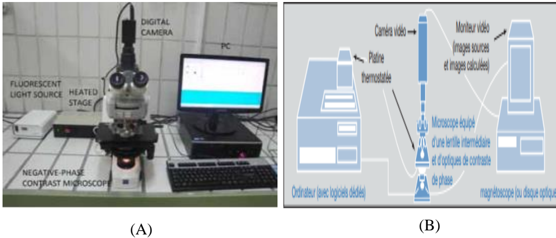
Figure 3: Equipment for Computer Assisted Sperm Analysis , (A): real picture(Michos et al., 2017) ; (B): Schematic of CASA.
