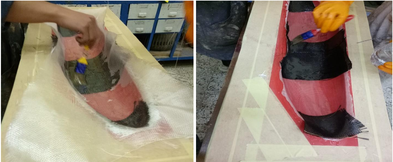
Fig (IV.18). Applications of different fabrics for molding.
