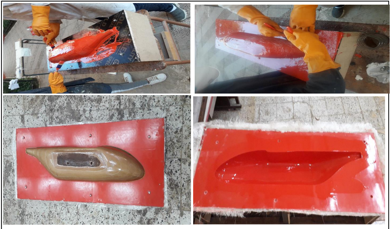
Fig (IV.17). Application of Gelcoat and the realization of the 1st shell.
