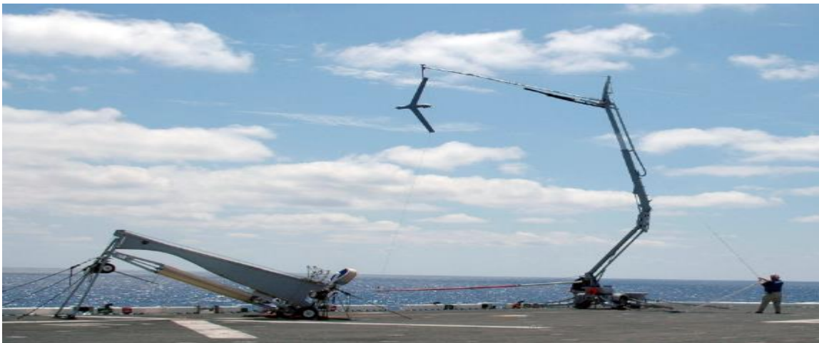
Fig (II.30). Suspended cable recovery
