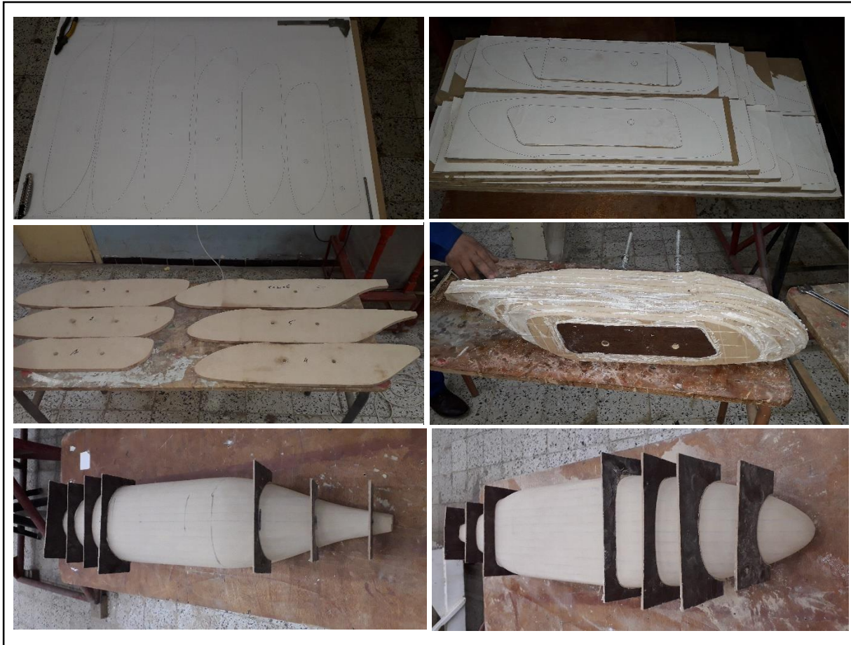
Fig (IV.8). Fuselage construction steps.
