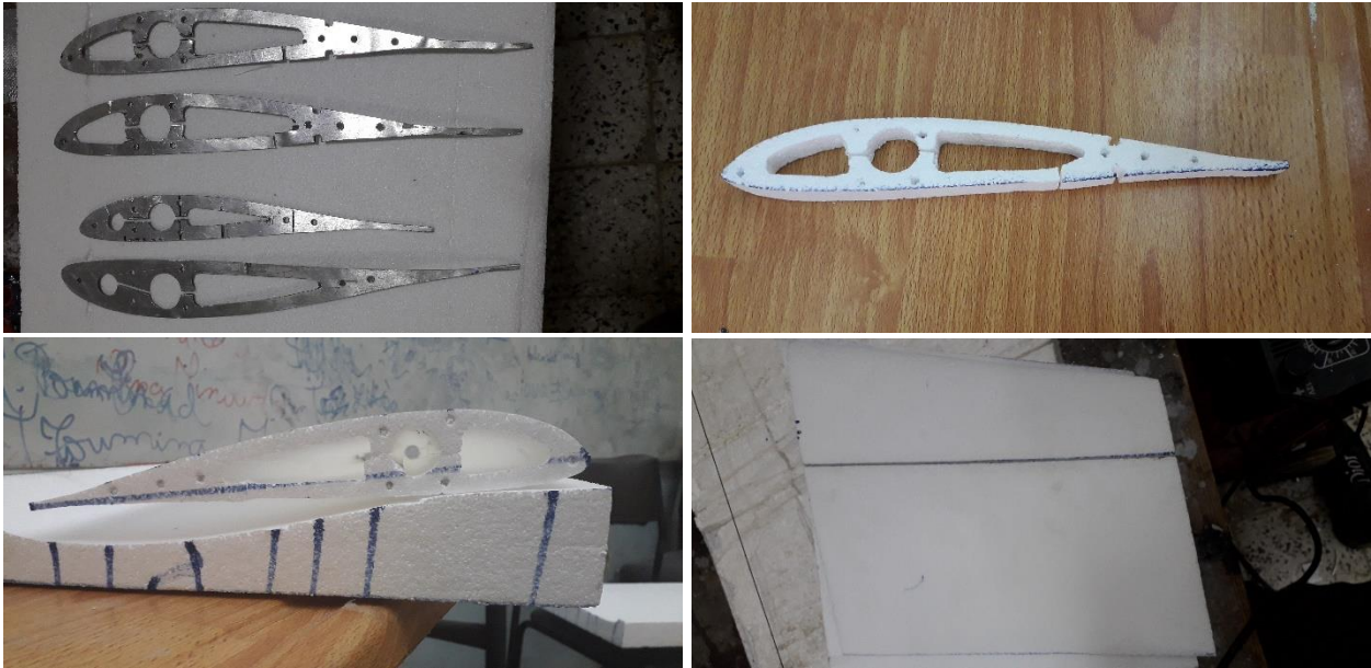
Fig (IV.9). Wing and empennage fabrication steps.
