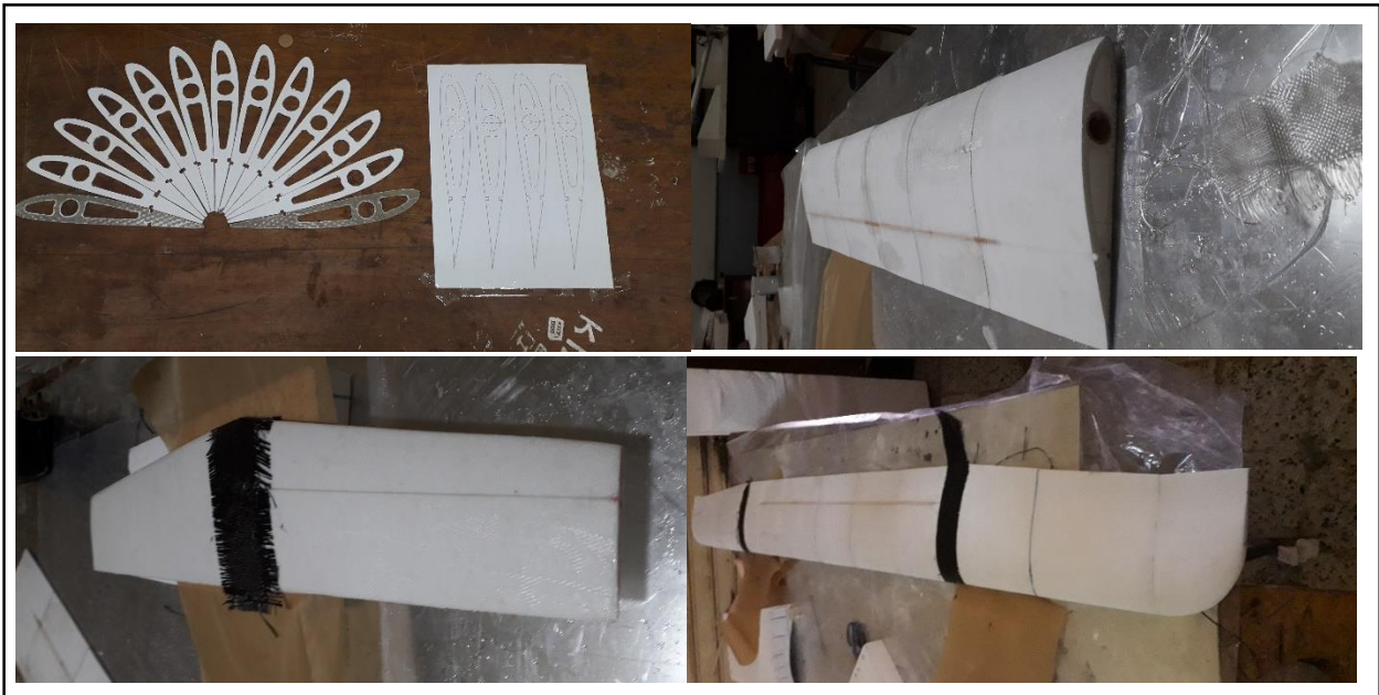
Fig (IV.14). Different steps for strengthening
