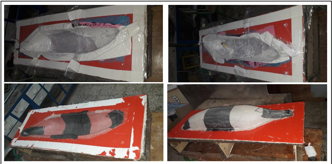
Fig (IV.19). Application of the vacuum pump.
