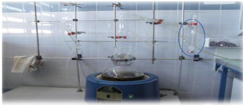
Figure 6: Montage d'hydro distillation (clevenger) (J.Smadja, 2009)
