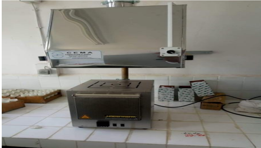
Figure 18 : Photo de four a moufle (original,2020)
