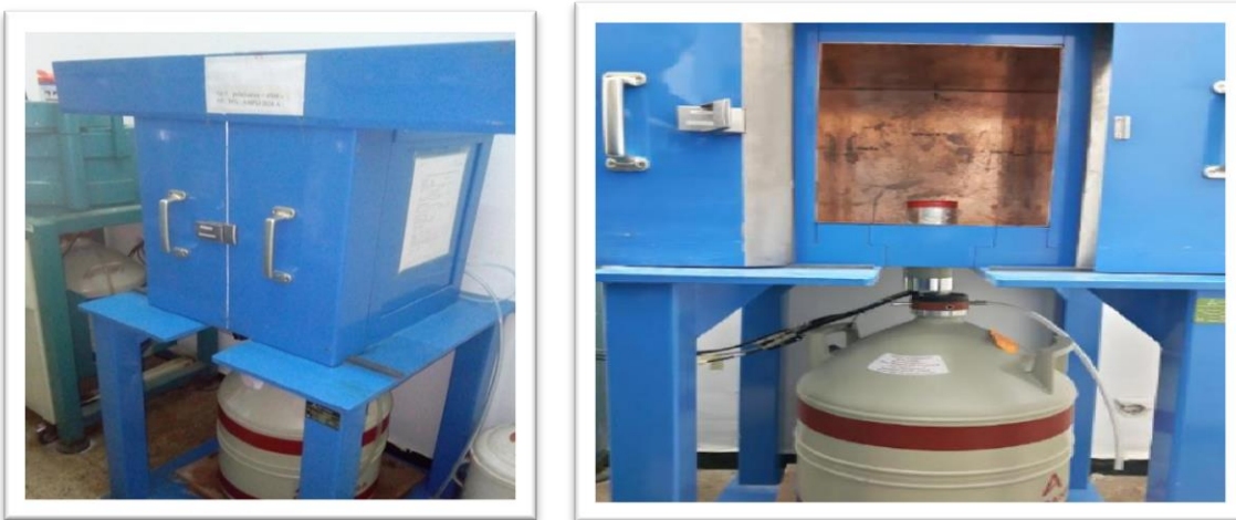
Figure III.2: Ge(HP) type semiconductor detector with coaxial geometry mounted on a vertical cryostat maintained at the temperature of liquid nitrogen
