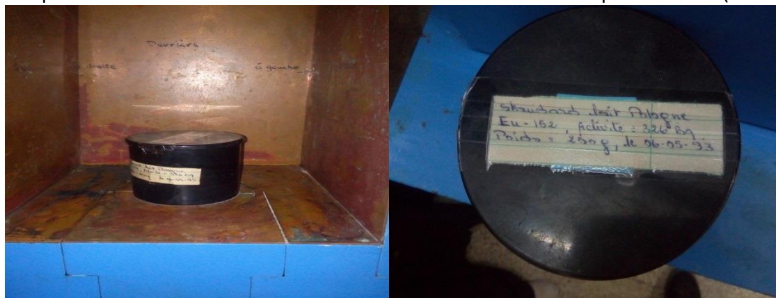
Figure III.5: Standard sample used for calibration in efficiency
