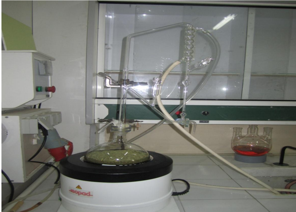
Hydrodistillation montage Clevenger.
