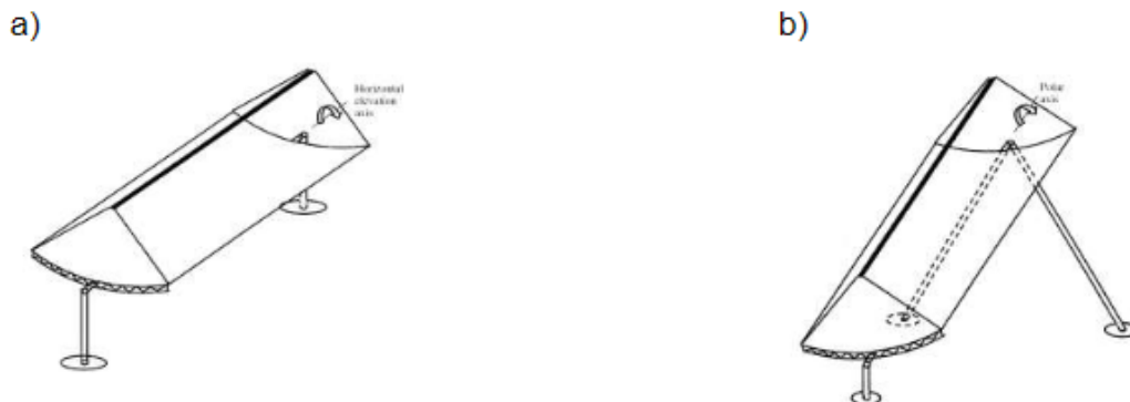
Fig.3.7(a,b): One-axis tracking configurations: a) One-axis horizontal tracker with reflective trough; b) One-axis polar axis tracker with reflective trough [20].
