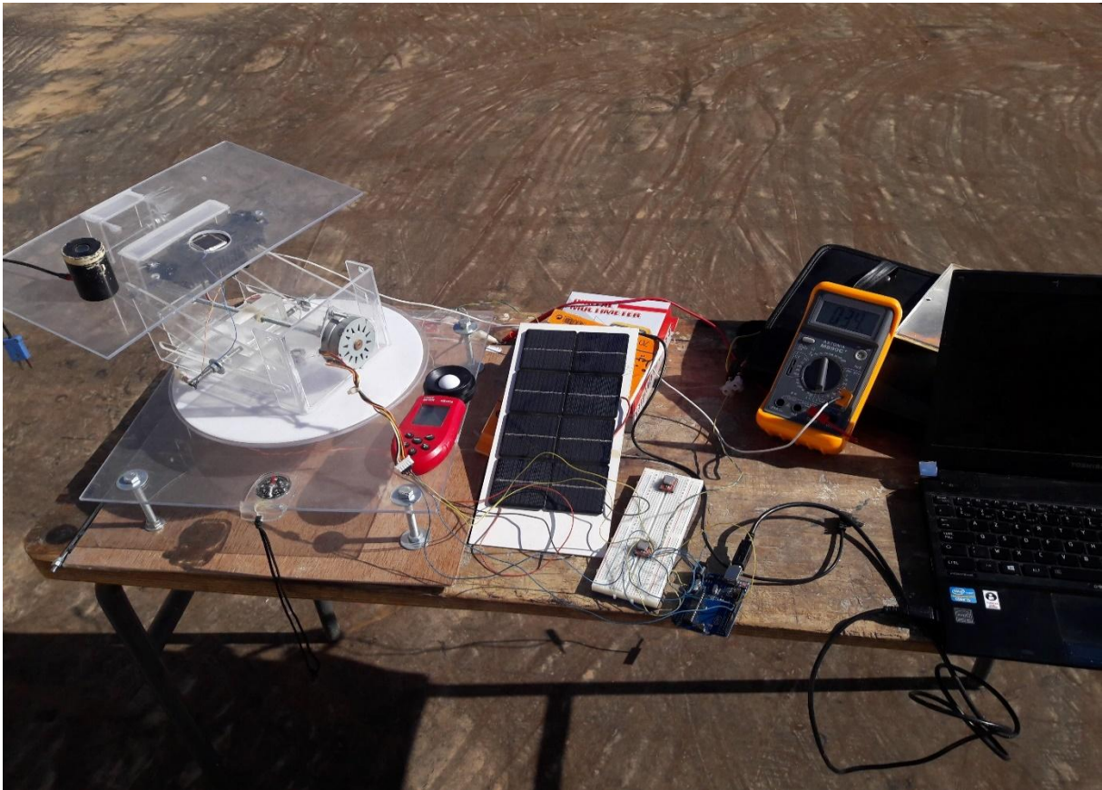
Figure.4.1: The sun tracker and the solar cell employed in the tests.
