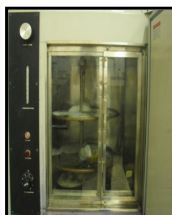
Figure 36: Etuve de conservation des lames
