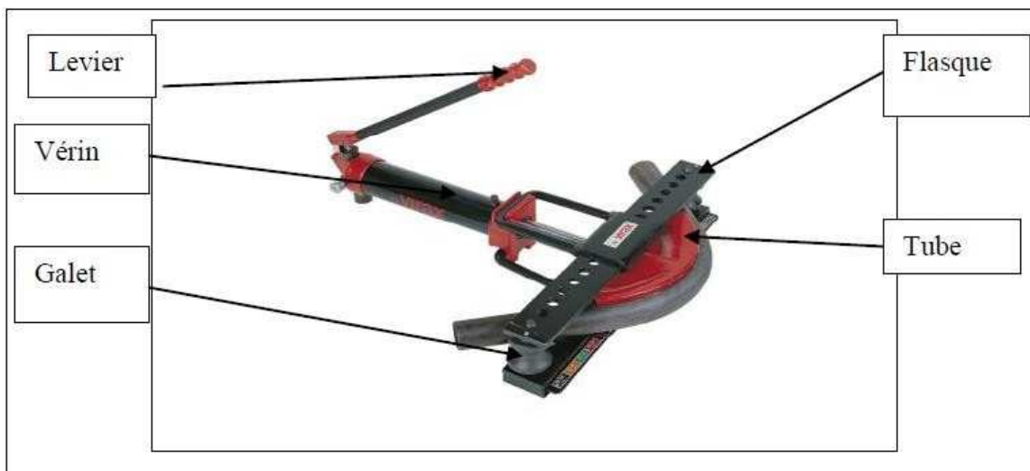
Figure II.6: Cintreuse hydraulique manuelle. [7]
