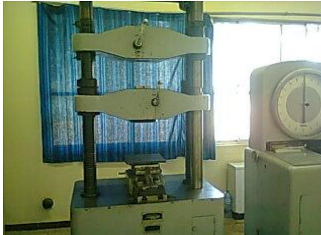
Figure 3 - 21 Machine de traction type RH-50 (SHIMADZU)
