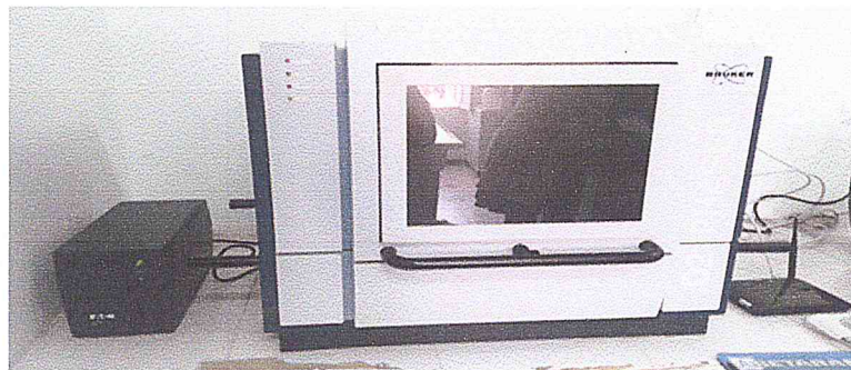
Figure II.3: DRX (Burker D2 Phaser).
