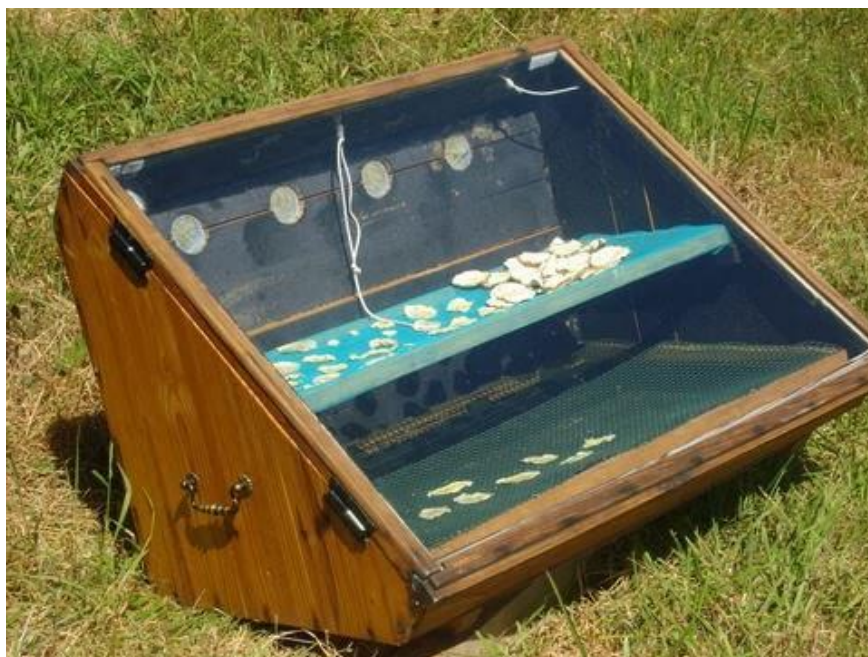
Figure 13:Le séchoir solaire coffre [66]
