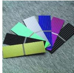
Figure IV.5: Cellules colorées monocristallines
