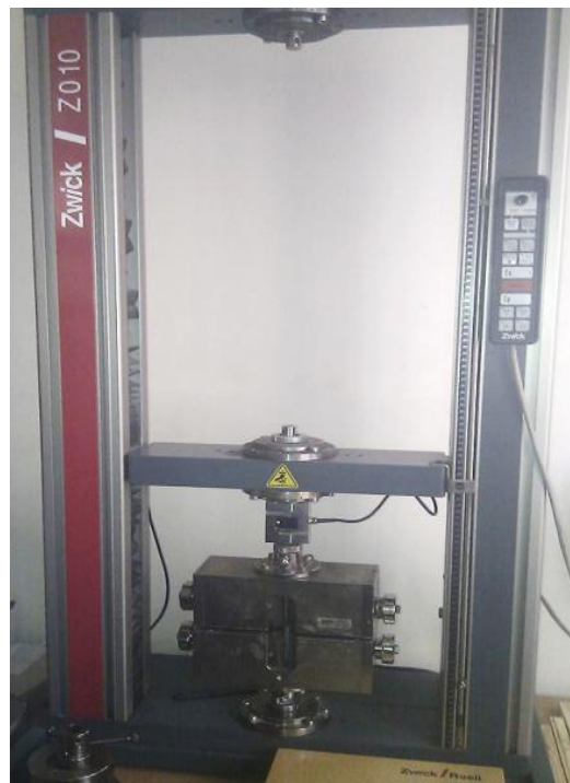
Figure II.28 : Machine universelle de compression de type ZWICK/ROELL Z10
