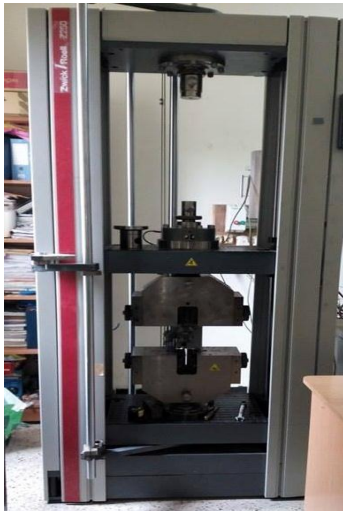
Figure II.23 : Machine universelle de traction de type ZWICK/ROELL Z250
