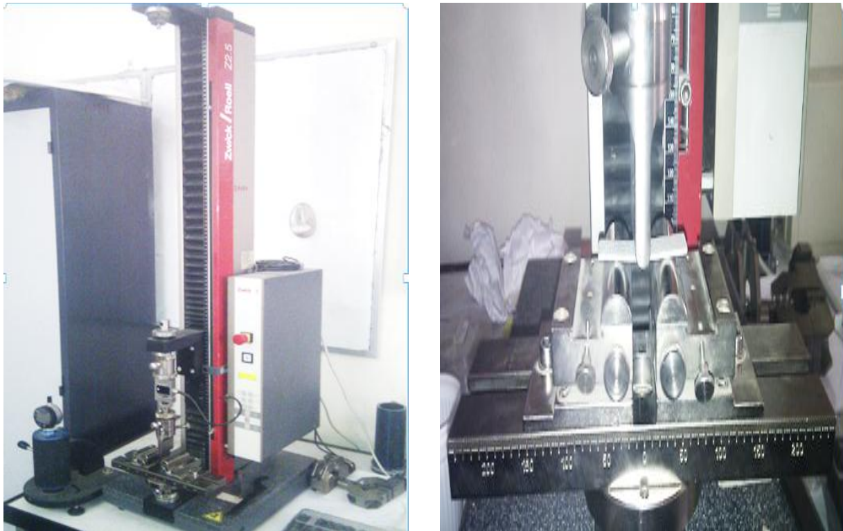
Figure II.26 : Machine universelle de flexion de type ZWICK/ROELL Z2.5
